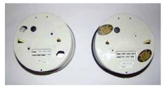
AutoMeter 5 inch Series I and Series II tachometers (left) and speedometers (right) have a LAMP terminal in the 8 cavity gauge connector. Series II gauges (on the right) require the light power lead to be on this terminal. Series I gauges (on the left) use separate light sockets and the LAMP terminal is not functional. Refer to the enclosed light socket connection photo to connect these sockets.
